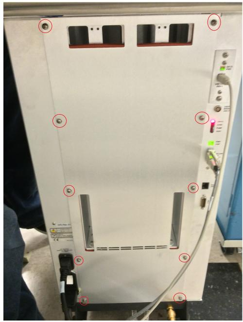
4. Unplug the affected cable assembly from the back side of both power entry modules and the line filter, a total of six connections).
