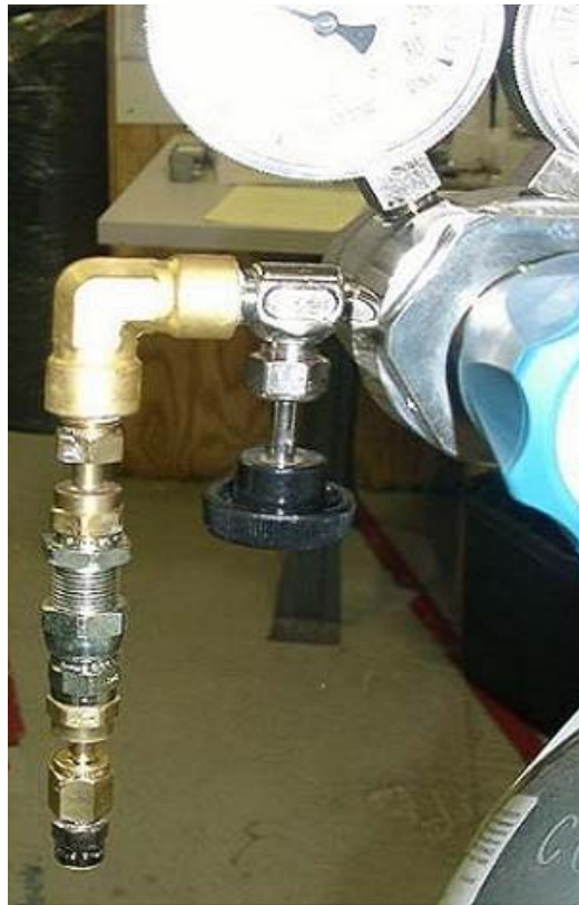
Figure 3. *Note Using only one wrench to remove this fitting can cause damage to the Gas Tank Regulator Relief Valve Assembly (4095-243).
