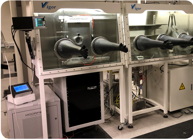
MiniLab 090 system with thermal evaporation and magnetron sputtering techniques
