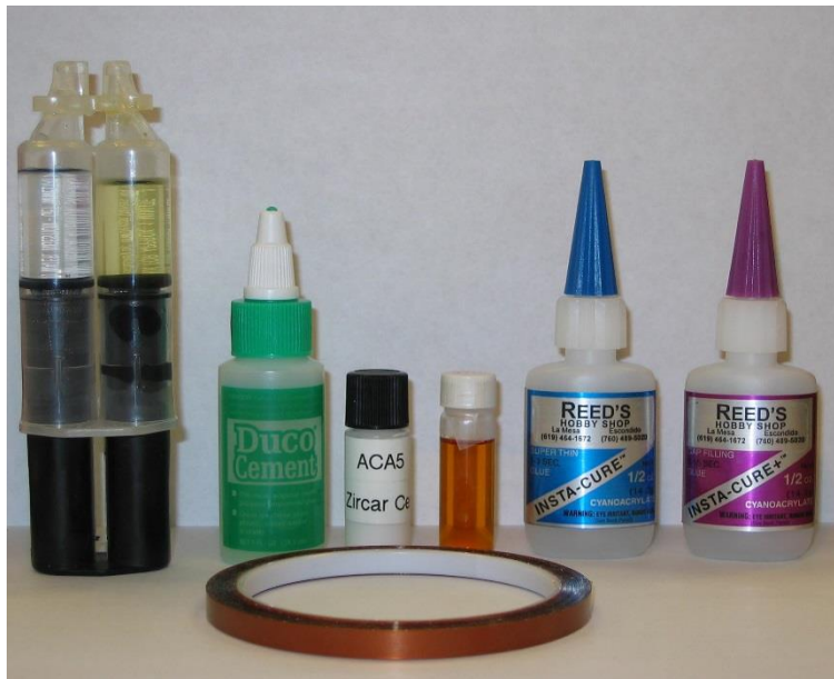
Securing agents from the left: 2-part epoxy; Duco cement; Zircar Cement; GE7031 Varnish; fast curing Superglue; slower curing Superglue; Kapton tape.
