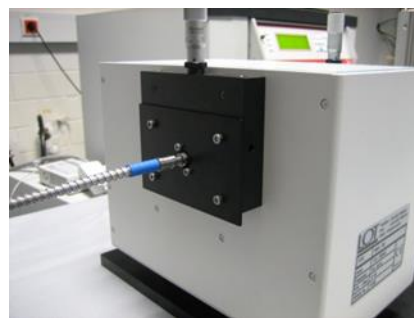
Figure 5: The fiber end is just screwed to the output of the monochromator. This monochromator has a variable slit width. For easy handling and more robustness, a commercial unit will have a slit with a fixed width.
