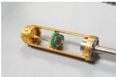
Figure 3: Sample part of the MFP with a commercial photoresistor.
