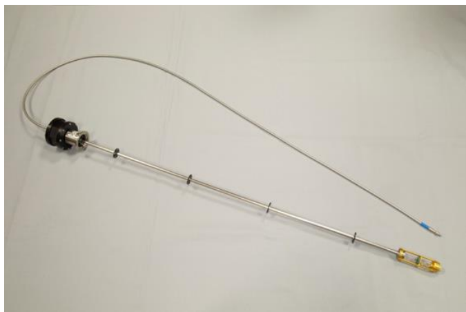
Figure 2: Fiber installed to MFP. Fiber outlet inside MFP case: polished circular surface perpendicular to fiber. Fiber outlet protected and centered by an anti-magnetic alloy.
